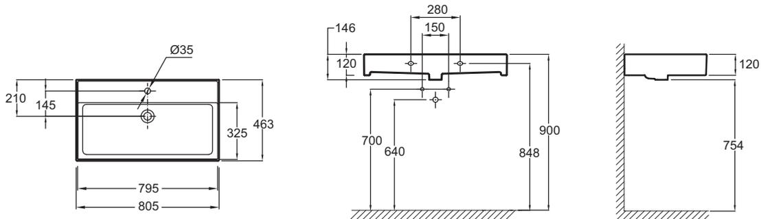
Product Specification: Vanity top 80 cm. EXBI112. Collection: VIVIENNE. DIMENSIONS: 80.50 x 46.30 cm. WEIGHT: 20.8 kg. MATERIAL: Ceramic. INSTALLATION TYPE: Self-supporting or can be mounted on a specific cabinet. TAP DRILLING: 1 tap hole. OVERFLOW: With overflow. NUMBER OF VANITY BASINS FOR VANITY TOPS: Single basin. RECOMMENDED BRASSWARE: Cüff. ADDITIONAL INFORMATION: Tap and waste not included.
